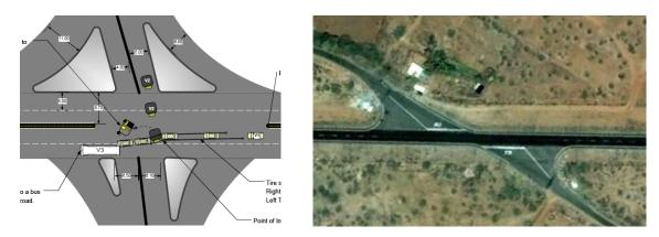
Figure 14. Intersections with Poor Road Alignments on the NH67 (Scene Diagram on the left) and NH47 Bypass (Google Earth Image on the right).
